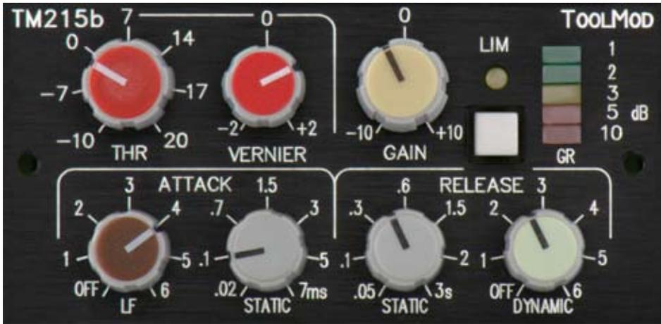
sical problem with limiting that is discussed below, the LONGEST PUMP FREE RELEASE TIME is the best possible setting. → Start with a release time of about 1.5 sec and go down until the pumping disappears.
