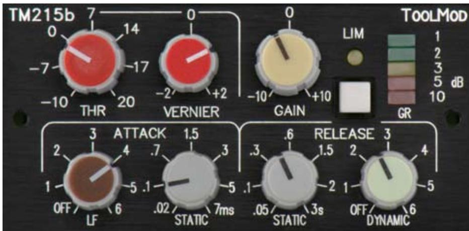
→ Set the dynamic release to the highest value that causes no pumping! Like the static release, the dynamic release increases the release time - in this case depending on the density of the signal - that may cause pumping. Usually you can reduce the static release time when you use dynamic release. Try both until you get the best possible compromise for the lf distortion without pumping.
