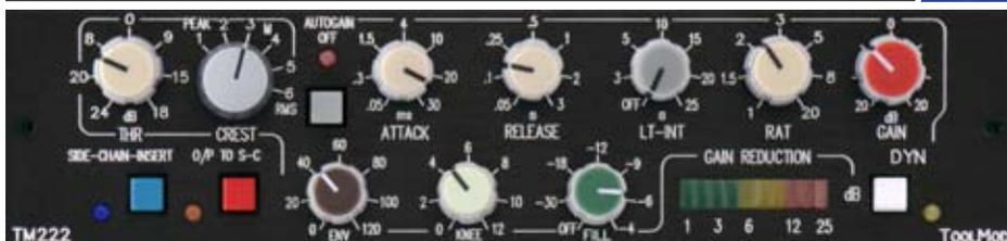
ve side effects. To keep the overall level constant, the threshold is shifted down with 'softer' knee settings. It's in the nature of things that the effect of a soft knee setting is lower if the ratio is small, since the difference between the uncompressed and the uncompressed range is small.
