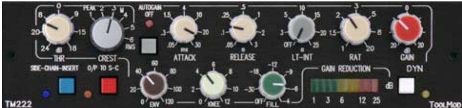
The TM222 Stereo Mastering Compressor comes with many additional functions to achieve high loudness gain without the typical 'compressor sound'. The module is best suited for mastering dynamics processing and as master compressor for mixing.
