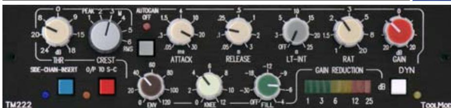
re that you don't have different levels with and without compressor for this test. The autogain should take care about this; however, you may need to fine trim the output level with the gain pot.
